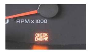
**Description:** An orange indicator light labeled CHECK ENGINE or SERVICE ENGINE SOON, it's also known as the MIL (Malfunction Indicator Lamp) in technical jargon. The importance and function of this light became more critical starting in 1996, when the second generation of onboard diagnostics, known as OBDII, became standard equipment on all makes and models of cars.
