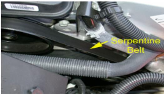
**Description:** Drive belts are made of reinforced, high-tensile strength cords and synthetic rubber. They connect the engine to front-mounted accessories. Belts come in two different types: The traditional V-belt (cross-section of belt has a V-shape) and the serpentine belt (also called Poly-V, Poly-Rib, Multi-Rib, and Micro-V belt), which uses multiple Vs for more positive contact with its mating pulleys.
