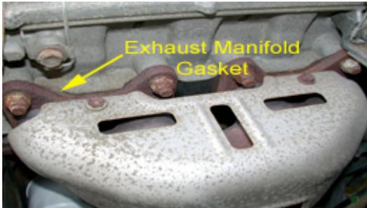
**Description:** Exhaust manifold gaskets may be made of embossed steel, sometimes in multiple layers. These gaskets may also be made of high-temperature fiber material, graphite, and ceramic composites, among others. Some gaskets use a combination of different materials. Other types of exhaust gaskets include flange gaskets and ring gaskets located at various connection points in the exhaust system. These gaskets are usually made from the same types of materials as exhaust manifold gaskets.
