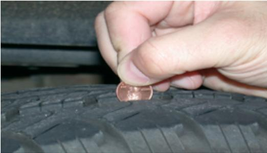
**Description:** There are several simple ways to check tire tread depth. The first way is to measure tread depth with a tread depth gauge. The second method involves the use of a penny inserted into the grooves of the tread. Tire wear bars are also used on today's tires as a hands-off visual indication that a tire needs replacement.
